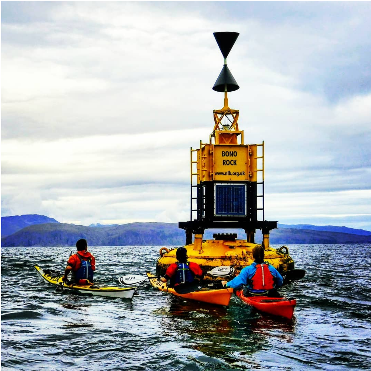
Figure 5.3: Bono Rock west cardinal buoy. The buoy marks the western extent of the Bogha Nuadh and Bogha Ghair reefs, south-west of Easdale in the Inner Hebrides. The eastern extent of the shallows is marked by the Bogha Ghair east cardinal buoy.
